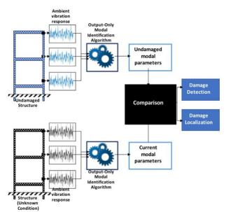
Fig -1: A schematic of output-only parametric vibration-based damage detection methods [32]
